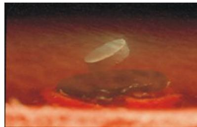
For the Meißner-Ochsenfeld-Effect the magnet is laid on the sample at room temperature. According to classic laws, no floating should happen as the magnetic field does not change any more. But after cooling the sample the magnet will float. This shows that superconductivity is more than perfect diamagnetism.
