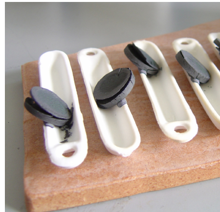
Superconducting pellets produced at the University of Munich for testing at teacher seminars, etc.
