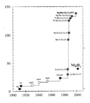
Figure 3. The history of the critical temperature for superconductors
