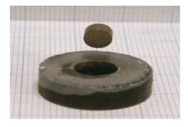
Figure 5 Levitation of a magnet over a superconductor.
