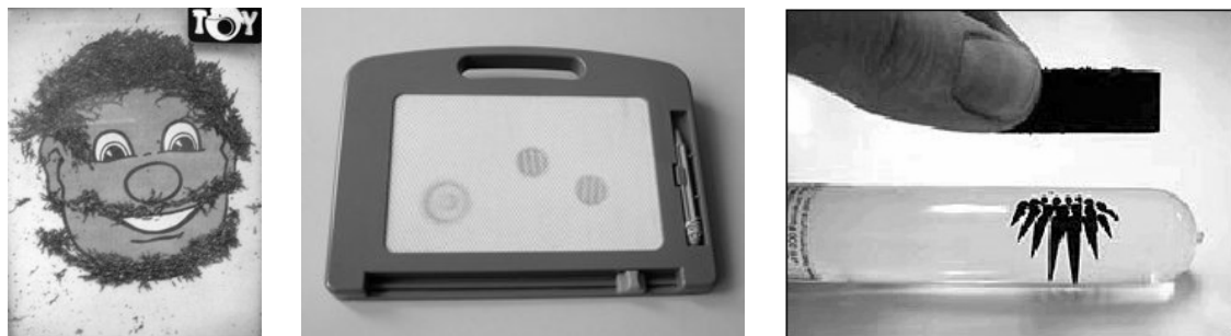
Fig. 6. Three devices to show the magnetic field lines. a) and old play with sub-millimetre iron filings, b) a novel screen for drawing for children, made of micro fillings suspended in paraffin oil; c) Ferro fluid cell [photo – www.teachersource.com ]
