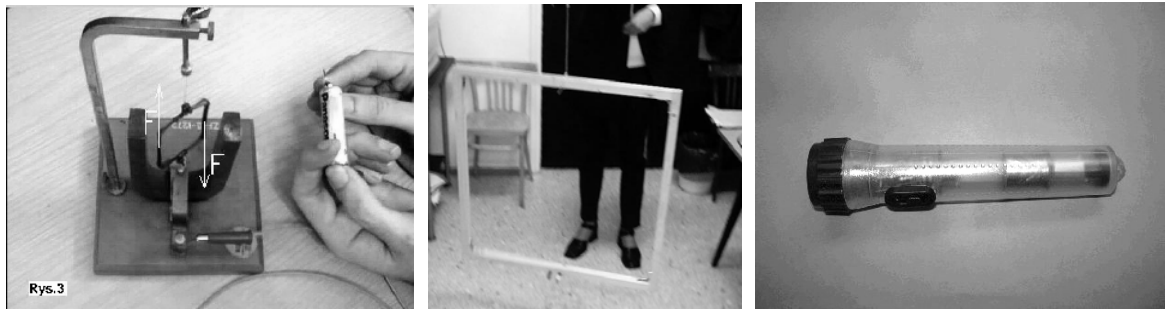
Fig. 3. AC current sources, or electric motors: a) a turning coil from the school lab [6], b) Helmholtz's coil - about 100 windings of 0.8 mm diameter wire (the chair and Ania's legs in the background are not necessary) c) hand-shaken lamp – the current is generated moving a magnets incite the coil (made in China).
