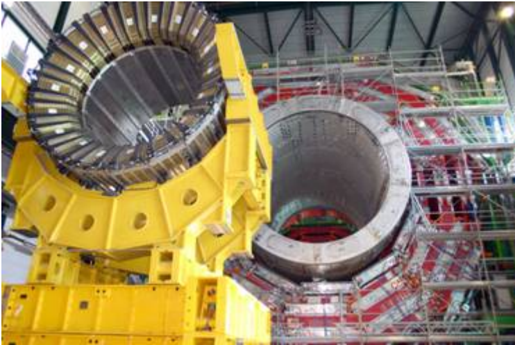
Superconducting solenoid, a part of the detector CMS within the LHC (Large Hadron Collider) at CERN http://en.wikipedia.org/wiki/Image:HCAL_Prepared_for_ionization.jpg
